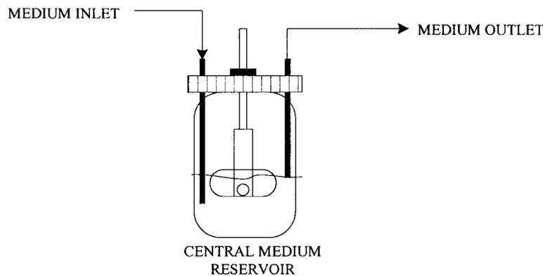
Fig. 4. Schematic diagram of a stirred bioreactor system.
