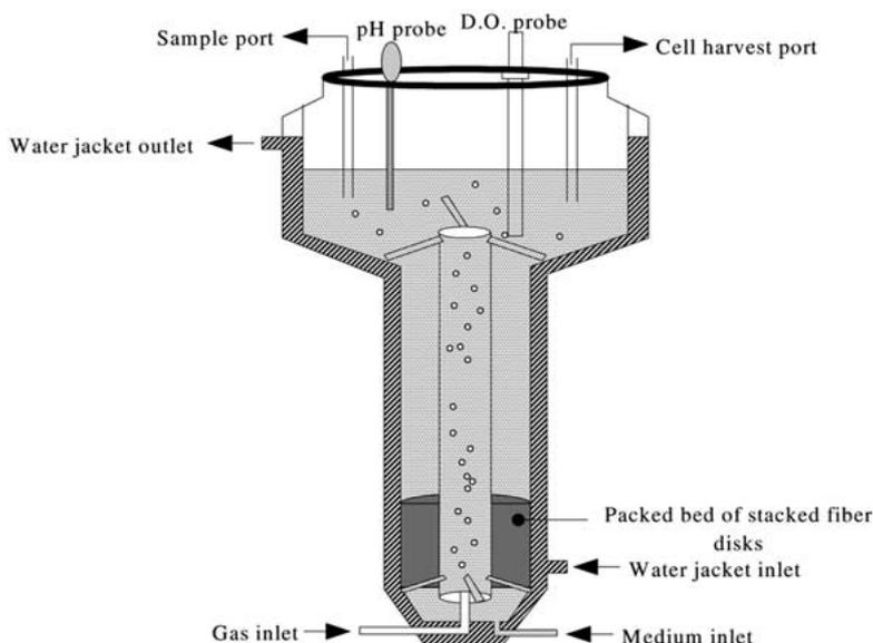
Fig. 6. Schematic diagram of an airlift packed bed bioreactor (adapted from Highfill *et al.* 1996).
