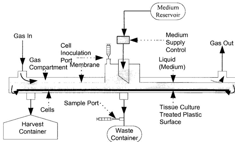
Fig. 2. Schematic diagram of the Aastrom perfusion bioreactor (adapted from Mandalam *et al.* 1999).
