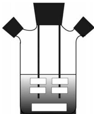
Fig. 5. Schematic diagram of a spinner flask.
