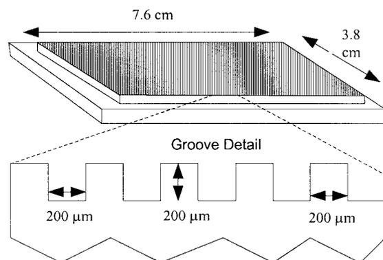
Fig. 3. Schematic diagram of a perfusion grooved culture chamber (adapted from Horner *et al.* 1998).
